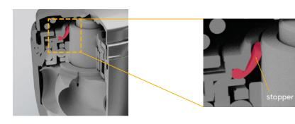
When the air supply is started, the rubber stopper floats due to the increase in air pressure inside the head. When the air supply is stopped, the stopper touches the rotating shaft and brakes.
